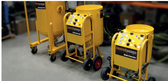
LEFT: EnviraSponge abrasive is available in a wide choice of grades to suit many different applications ABOVE: Sponge blasting on shipping container to demonstrate the low-dust produced RIGHT: Media generators from EnviraSponge sized from 100 to 500 liters
