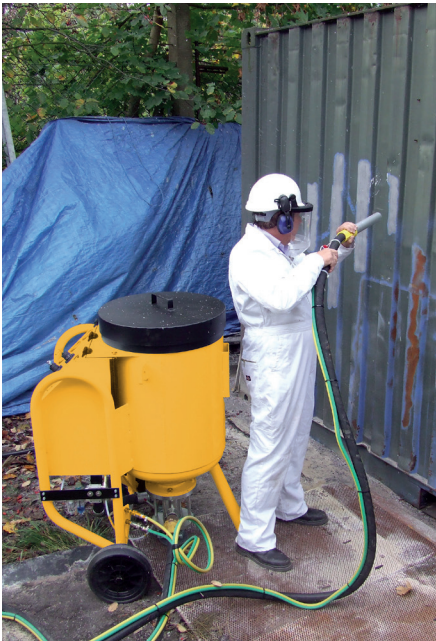
LEFT: EnviraSponge abrasive is available in a wide choice of grades to suit many different applications ABOVE: Sponge blasting on shipping container to demonstrate the low-dust produced RIGHT: Media generators from EnviraSponge sized from 100 to 500 liters
