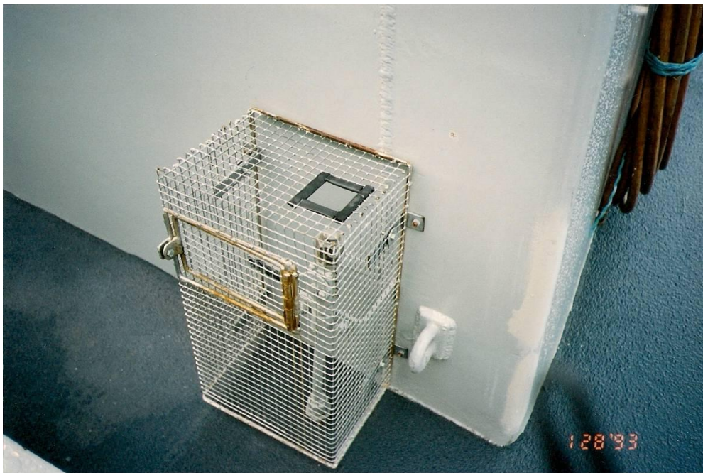
Figure 3.4 Plasticised Wire Mesh Breaking Down With Use
