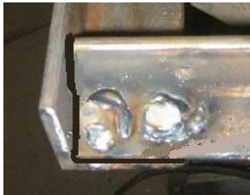
Figure 3.13 Filled Tack Weld
