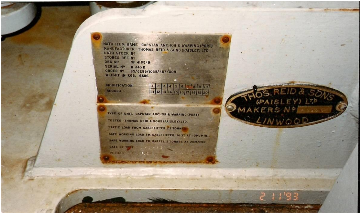
Figure 3.5 Manufacturers Nameplate with incorrect Fasteners
